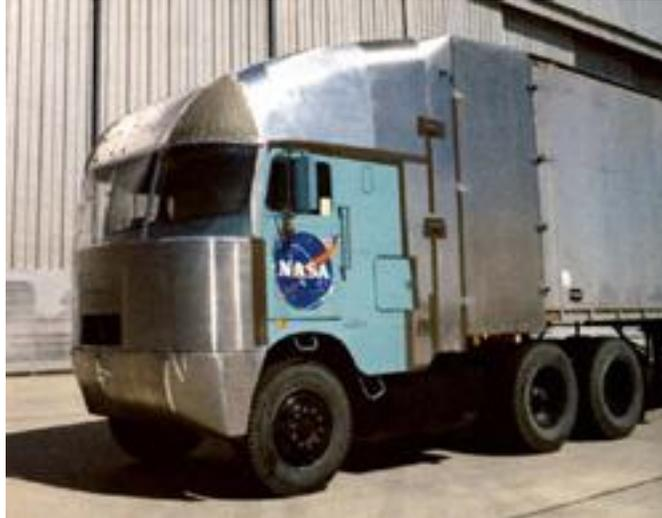
**Figure: Aerodynamic design for a truck cab**
