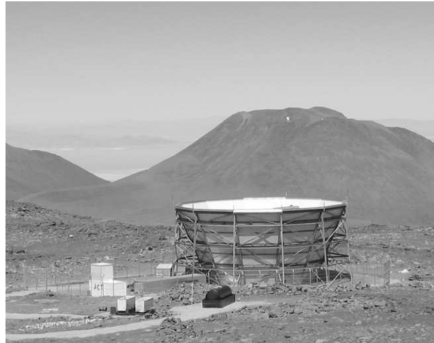
Figure 1. The Atacama Cosmology Telescope. Left: Drawings of the telescope. The full height of the telescope is 12 m. The entire upper structure (“azimuth structure” and above) rotates during scanning motion. The focus of the secondary mirror is below the primary mirror in the receiver cabin. The telescope is surrounded by a ground screen to block radiation from the earth. Another ground screen is mounted on the sides of the telescope itself. Right: The telescope in the Atacama Desert in Chile. The generators, fuel tank and shipping containers for storage, equipment and office space also appear in this photograph.
